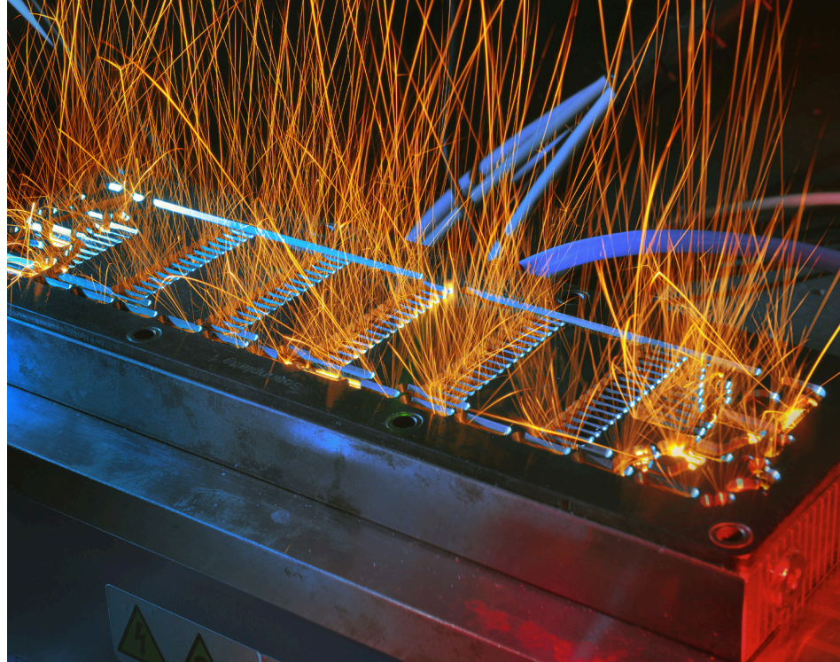
1 Setup with two RAYLASE AS-Fiber 30 scanners. 2 Welding a bipolar plate.
